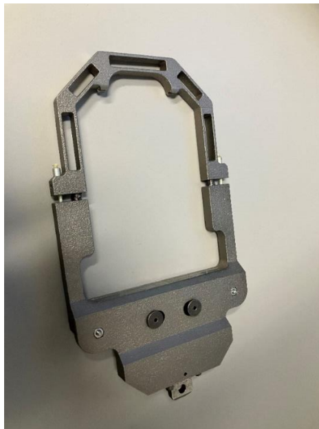
Figure 1: Robot gripper that has been manufactured with Ti-6Al-4V
